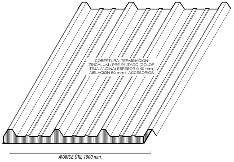
**ISOMETRICO DE THERMOPANEL**
