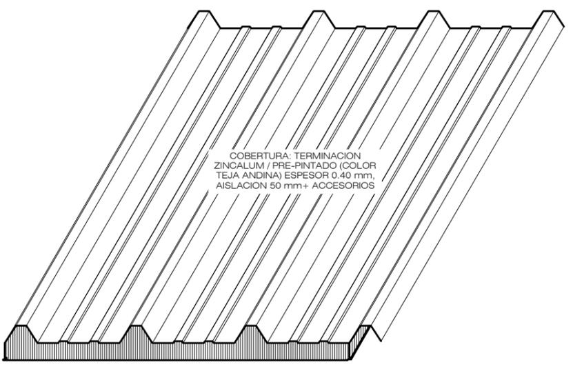
**ISOMETRICO DE THERMOPANEL**
