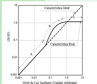
Graph of typical behavior of a PMT. The region A is the behavior of ideal (linear), the region B is the non-linear region and the C region is the region of saturation.
