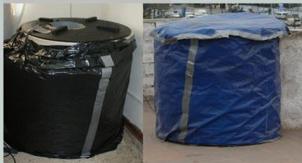
Commercial tanks used to construct Cherenkov tanks. It shows the external coating of polyethylene and the coating of blue plastic mesh for protection against the environment.
