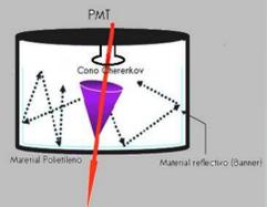
Outline of operation of the tank: A charged particle passing through the tank produces cone Cherenkov light, the light reflects off the walls to reach the lightsensor (photomultiplicador).
