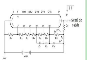
Typical diagram of the operation of a voltage divider: the voltage drop in the resistor R7 generated by the current  $I_p$  (due to light pulses) is offset by the decoupling capacitor C3, a similar situation occurs in R6 and R5
