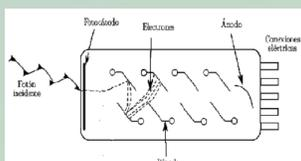
Outline of operation of a PMT, a photon strikes the photocathode releases an electron which is accelerated and is multiplied in the dynodes due to a constant potential difference between them.
