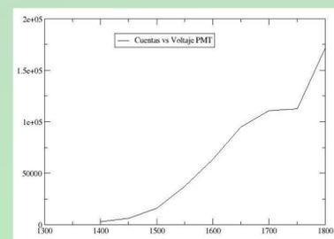
Flux at different voltage values used for the energy calibration of the Cherenkov detectors. The peak corresponds to a vertical muon that deposited 80 MeV.
