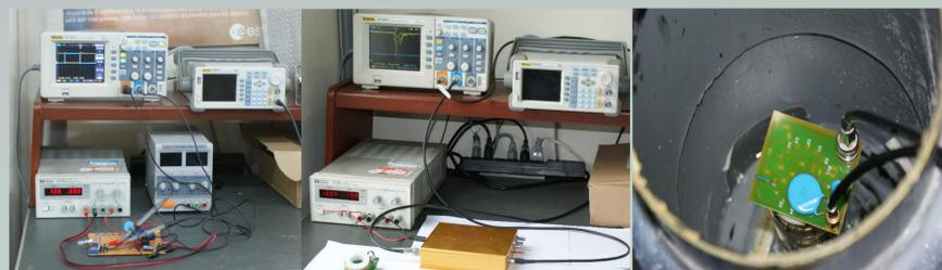
The pictures show: The bench test of the high voltage supply source without load (left). Full module operation: high voltage source, voltage divider and Cherenkov tank (center). The connections of the voltage divider in the Cherenkov tank (Right).
