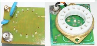
Voltage divider circuit assembly with surface components for the EMI 9530 PMT A.
