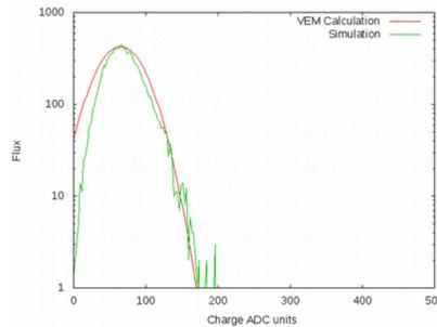
VEM charge histogram calculated from total charge and simulated (20000 particles).
