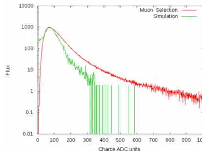
Muon selection charge histogram calculated from total charge and simulated (40000 particles).
