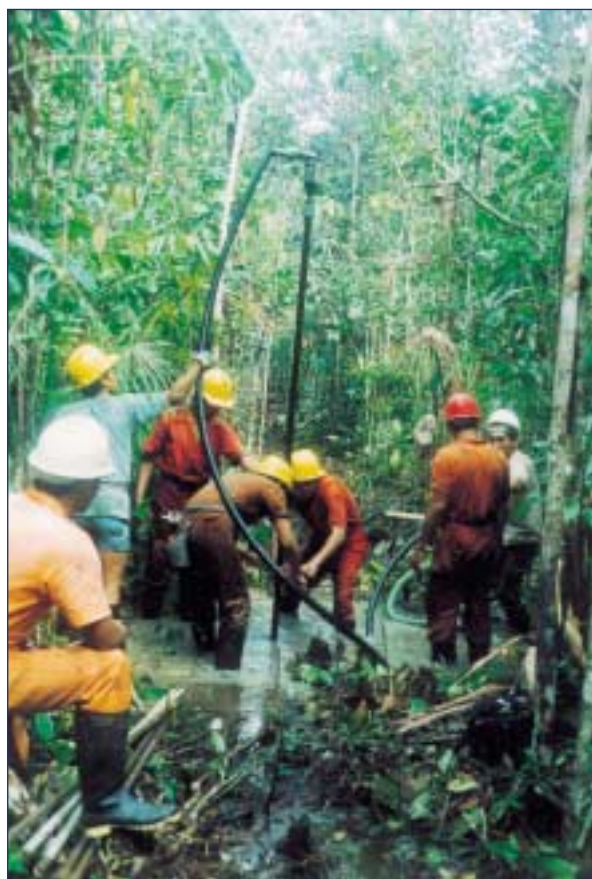
Colocando Explosivos para Registros Sísmicos - Selva Norte Explosives are Being Placed for Seismic Registers - Northern Jungle
