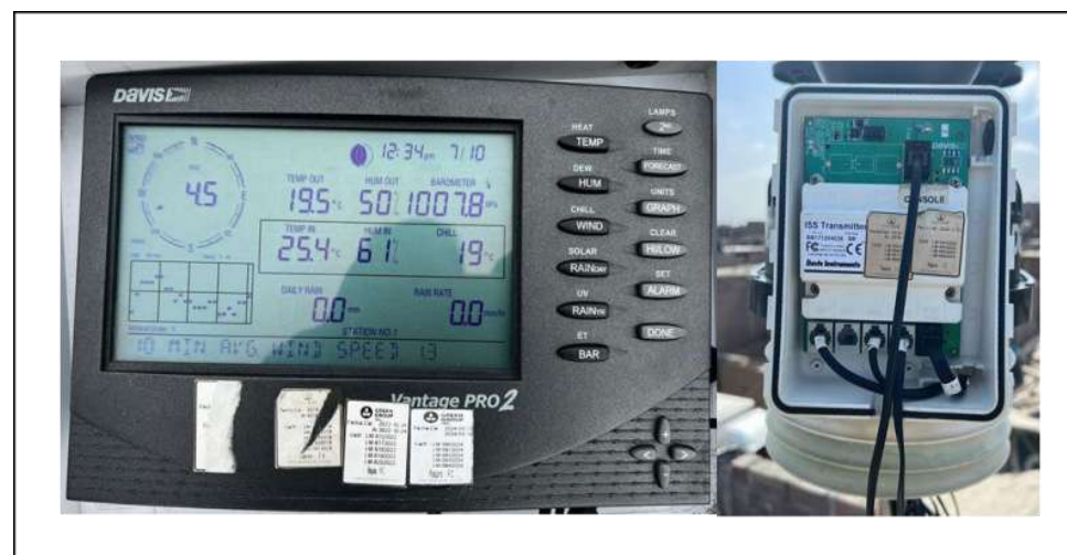
Figura 5. Data logger y Panel Integrated Set of Sensors (ISS)
